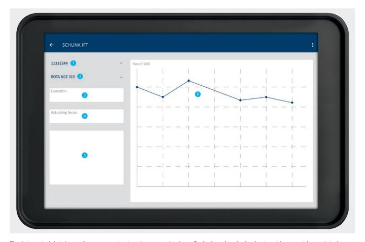
The integrated database allows access to stored measured values. Each clamping device is stored in a machine-related way. This allows the measured values to be visualized at any time via the app.
