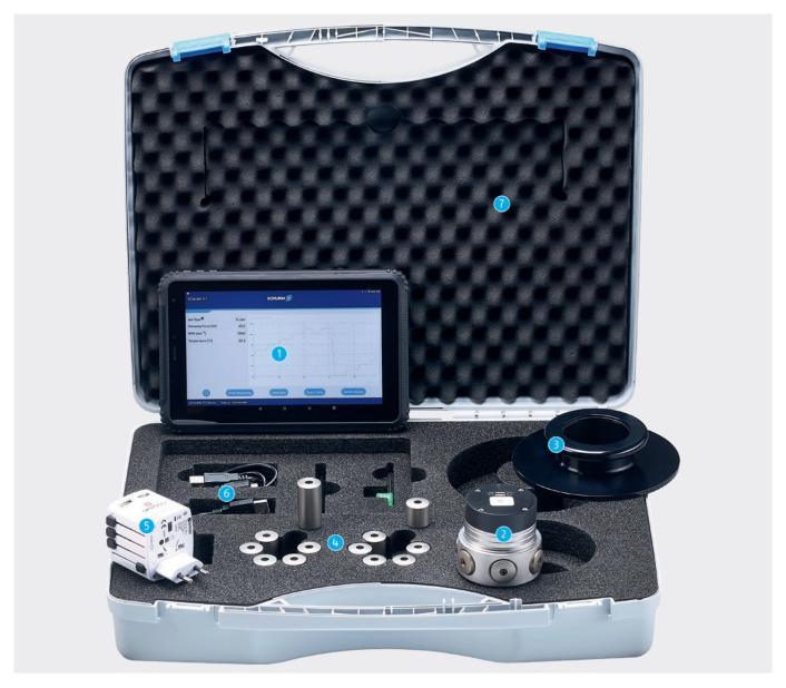
The IFT clamping force tester is delivered in a convenient yet robust case. The case contains all of the necessary tools for conducting clamping force measurements on the machine.
