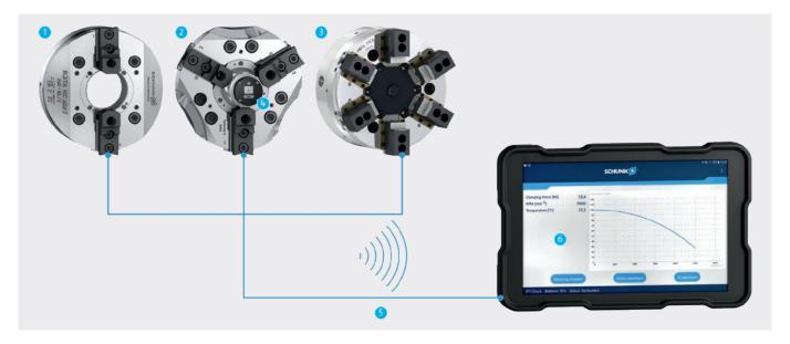
With the measuring head IFT-M1, clamping forces of 2-, 3-, and 6-jaw chucks can be measured quickly and with high accuracy. The measured values are transmitted wirelessly from the measuring head to an industrial tablet computer and displayed there in an app. In the integrated database, the measured values can be stored based on the relevant machine and chuck. These can then be called up again at any time, for example in case of maintenance.
